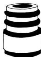
BRASS INSERT WITH O RINGS AND FIXED SEATING WASHER. X2 THESE PARTS ARE ALSO USED IF USING PARTS IN BOX B
