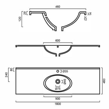
DIMENSIONS 1800mm length x 460mm width x 120mm depth
